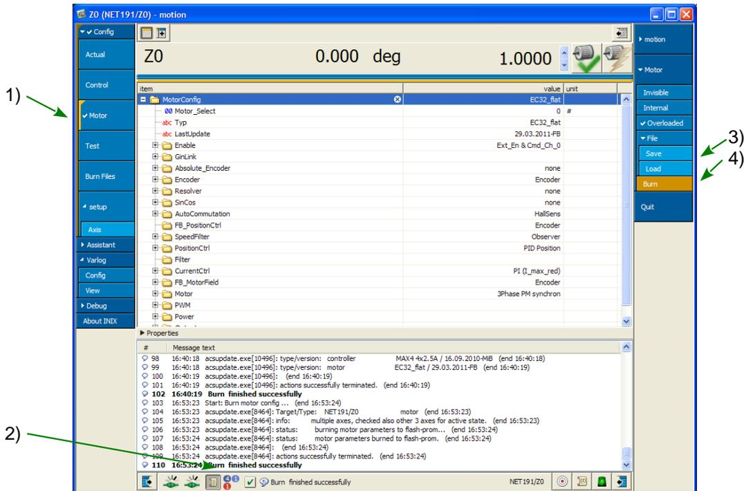
Fig. 4: Burning and saving motor configuration parameters
