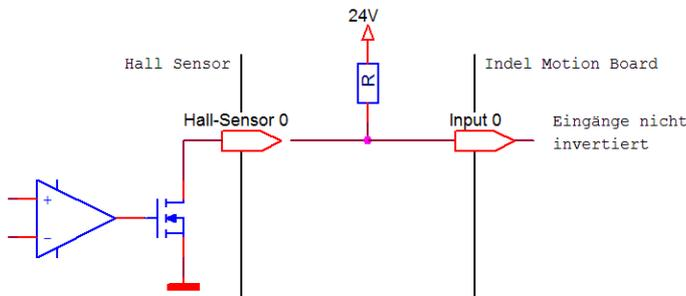
Fig. 27: Wiring with non-inverted inputs
