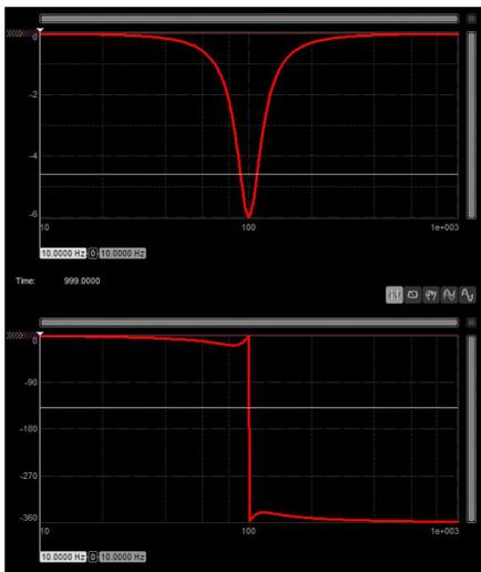
Fig. 65: Notch filter -6dB amplification
