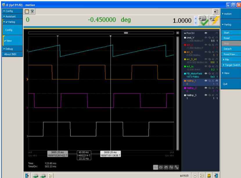
Fig. 30: Hall sensor sequence, standard direction of rotation CW
