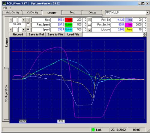
Fig. 79: Incorrect Ke; recording with speed waves
