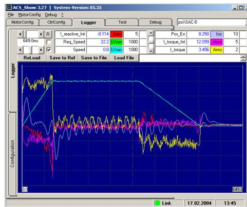
Fig. 80: Incorrect Ke; recording with active current-idle current-integral Image on left: incorrect Ke, image on right: correct Ke
