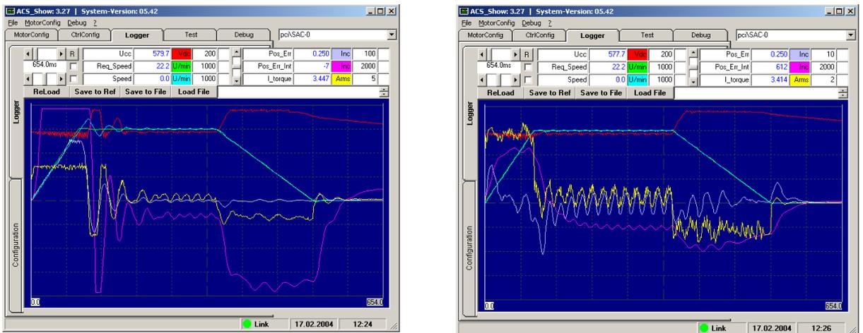
Fig. 82: Incorrect resolver offset; recording with speed waves Image on left: incorrect, image on right: correct resolver offset
