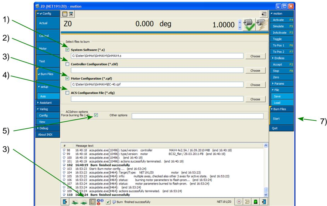
Fig. 3: Loading firmware, motor/controller configuration
