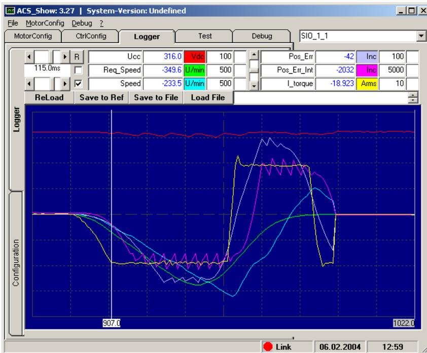
Fig. 84: Incorrect resolver offset, speed waves
