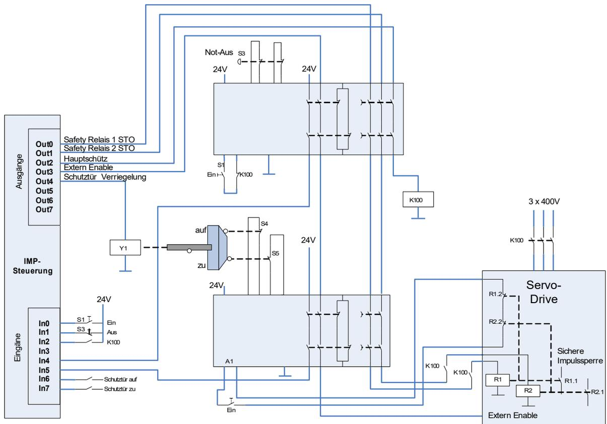
Fig. 46: Example: STO, locked safety door
