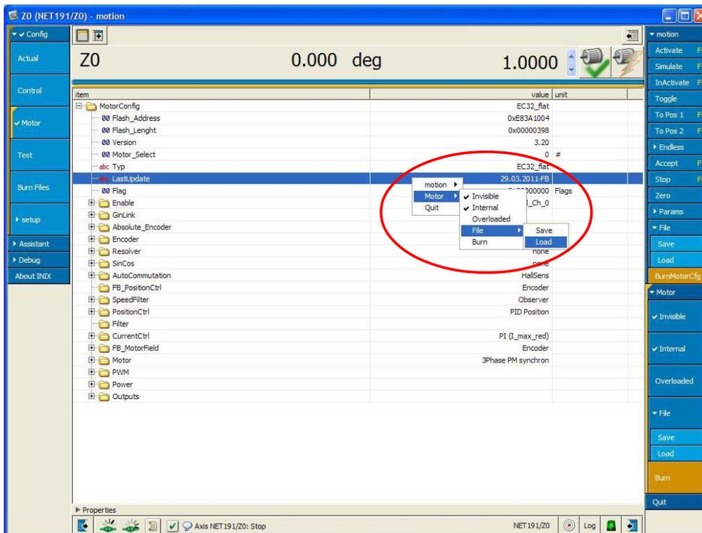
Fig. 5: Saving and burning motor configuration parameters
