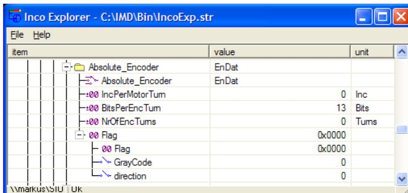
Fig. 10: Absolute encoder configuration
