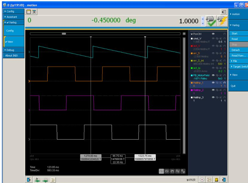
Fig. 29: Hall sensor sequence, standard direction of rotation CCW
