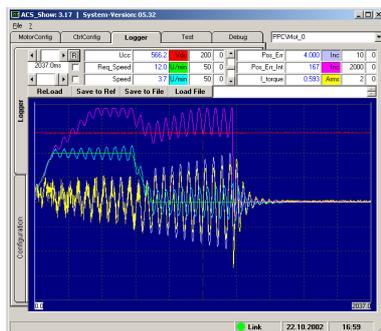
Fig. 55: Critical amplification  $kP_{crit}$  too high
