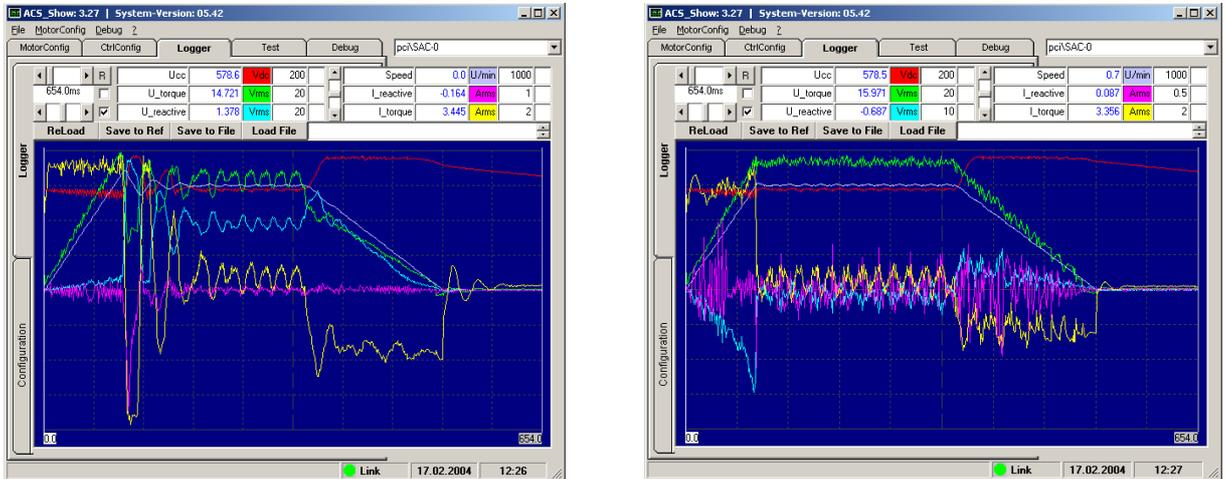
Fig. 81: Incorrect resolver offset; recording with voltage waves Image on left: incorrect, image on right: correct resolver offset
