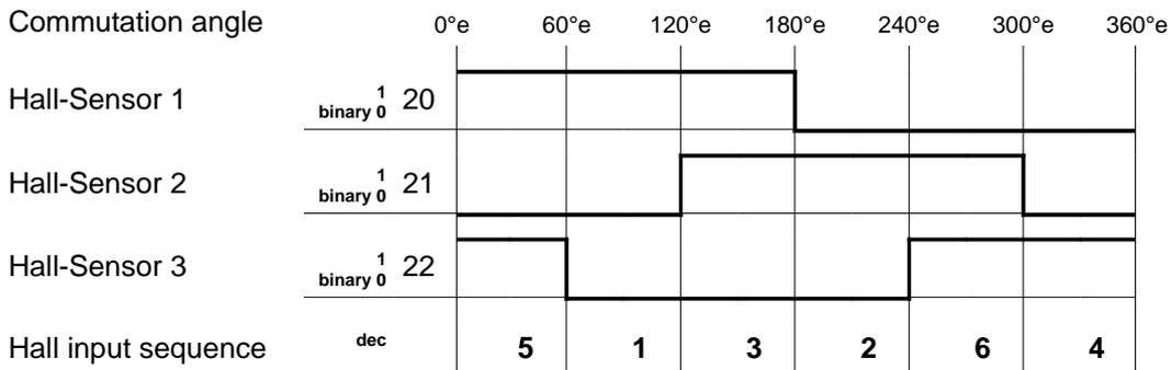
The commutation angle is given in field degrees (°e). Warning: in motors with more than one pole pair, the degrees on the motor shaft do not match the field degrees.
