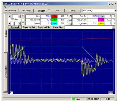
Fig. 57: *kP* was increased until the current and following error vibrate again
