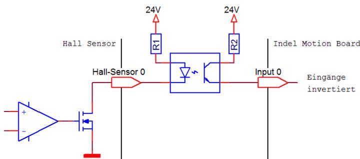
Fig. 28: Wiring with inverted inputs
