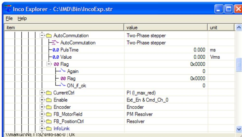
Fig. 23: Auto-commutation Two-Phase Stepper
