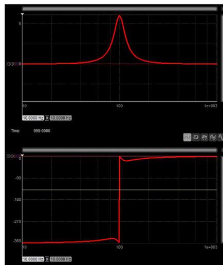
Fig. 66: Notch filter 6dB amplification
