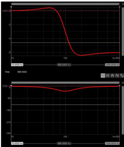
*Fig. 62: Low-pass filter -6dB amplification*
