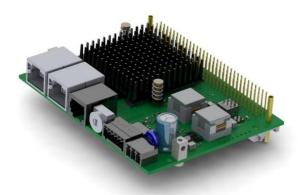
customer-specific electronics, etc. If the master COP is used as a fieldbus slave, it serves as an active bus coupler with its own CPU. The decentralised computing power can be used for signal pre-processing and the execution of customer-specific algorithms.
