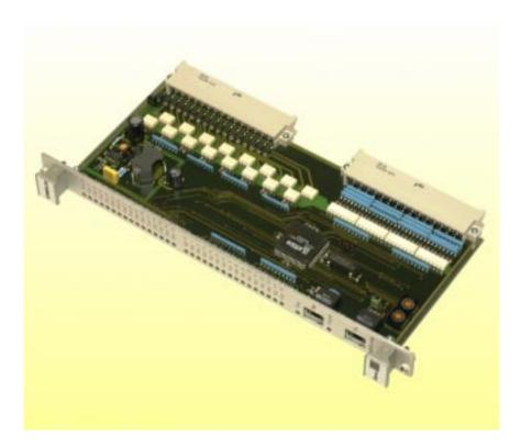
The INFO-I16r board differs from the other I/O boards in that its inputs and outputs are individually isolated. All inputs and outputs can be connected as required to plus or minus. The board is an ideal replacement of relay
