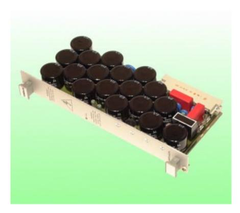
The power supply INFO-ACPr generates the 325VDC intermediate Voltage required by the INFO-ACSr servo controllers. The card is protected against overvoltage and overcurrent. At most ten servo controllers INFO-ACSr-6A/ 10A or five INFO-ACSr-20A can be supplied.
