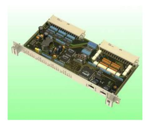
The INFO-4KPr is the field bus node for high-precision and very fast positioning and control tasks. Four complete and independent channels are incorporated on the board.
