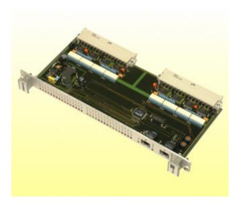
The INFO-32Or board belongs to the digital I/O modules; as all modules, it is serv-ed once per millisecond, i.e. each input and each output in the machine or plant is refreshed everyms. The power supply of the outputs is
