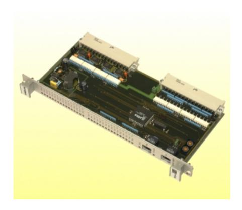
The INFO-16Pr board belongs to the digital I/O modules. As all modules, it is served once per millisecond, i.e. each input and output in the machine/plant is refreshed every ms.
