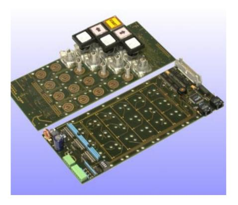
The INFO-TSP board includes a keypad combined with a parallel interface for activating an LCD display.
