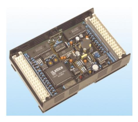
The INFO-FADC board (Fast Analog/Digital Converter) is the measurement element for the registration of fast and dynamic processes.
