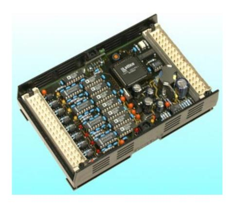
The INFO-DAC board outputs 8 voltages of  $\pm$  10V or currents of 0 ... 20mA with a resolution of 16 bit.
