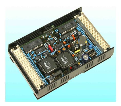
The INFO-ADC board is the measurement element for the precise measurement of analog quantities.
