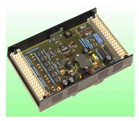
The INFO-4KP is the field bus node for high-precision and very fast positioning and control tasks.
