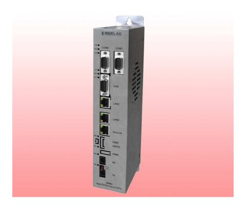
The GinLink Stand Alone Master board is the field bus master of a GinLink. The board operates entirely autonomously and does not need any higherranking computer for operation. for visualisation and software updates, a 1GBit Eternet port and two RS232 interfaces are available.
